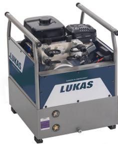
The powerful power units of the 650 series supply all your devices from the LUKAS rerailing system with the necessary power for your project. The use of two- or also four-flow radial piston pumps is possible. Depending on your needs, up to four hydraulic cylinders can be supplied with the same flow rates. Maneuver synchronous extension and retraction of identical lift cylinders via the control desk. The gasoline gensets are equipped with pull-rope starters and electric starters.
