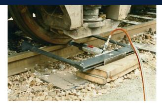
If the vehicle wheels are on the rail with the wheel flange, the axle pusher presses them into the track. You will also need the LFM 10/160 cylinder and the matching piston protection plate.
