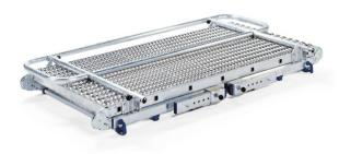
The device consists of an aluminium platform equipped with a foldable ladder on each end. The ladders have adjustable feet which can be used to level out uneven surfaces. A guardrail can be inserted on both sides of the basic platform. The device can also be used on rails by fitting a separately available set of wheels (not included in the scope of delivery).
